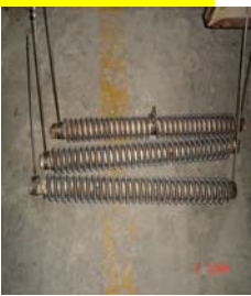
Coil wire around tube
